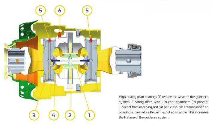
The central lubrication system (3) supplies the joint adequately with lubricant. The joint crosses are fitted with the blue "P" seal(4). The cap bottom lubrication (5) and the double-fork direct lubrication (6) help make the lubrication process easier.
