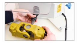
**Assembly and dismantling**Minimum force required for dismantling and assembling the joint
