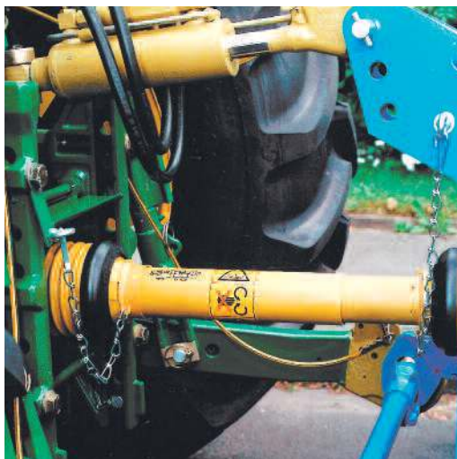
The PTO drive shaft correctly secured with two safety chains
