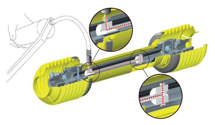
With the new Profile Tube Lubrication System, GKN Walterscheid responds to market requirements: Improved handling and minimised maintenance efforts.
