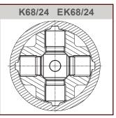
Walterscheid GmbH sets all clutches exactly to the specified torque. The spring assembly is preset in accordance with the required torque.
